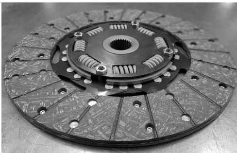
IMAGES DEPICTING TRANSMISSION SIDE OF CLUTCH DISC (EXC. 1993-97 F-BODY)
